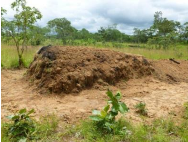
Figure 31- Traditional charcoal manufacturing
